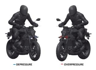
Due to its angles and frontal surface, it creates an overpressure on the top of the spoiler. The turbulance create below, generates a difference of pressure between the upper and lower part of the spoiler. Which ultimately generates the aerodynamic downforce.
