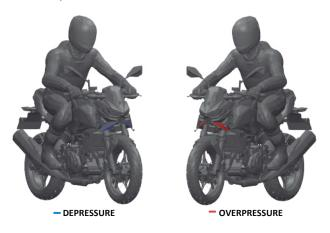
Due to its angles and frontal surface, it creates an overpressure on the top of the spoiler. The turbulance create below, generates a difference of pressure between the upper and lower part of the spoiler. Which ultimately generates the aerodynamic downforce.
