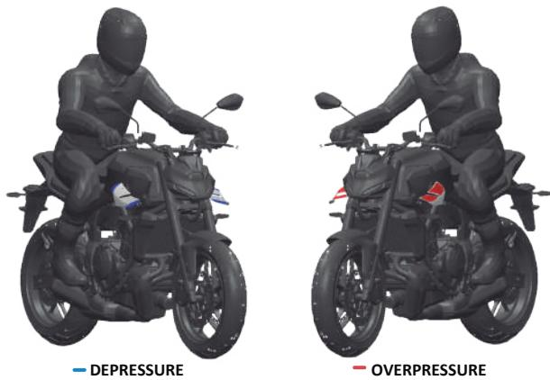
Due to its angles and frontal surface, it creates an overpressure on the top of the spoiler. The turbulence creates below, generates a difference of pressure between the upper and lower part of the spoiler. Which ultimately generates the aerodynamic downforce.
