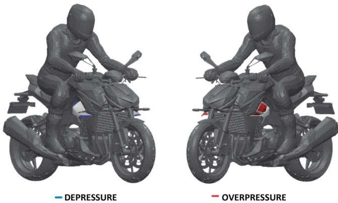
Due to its angles and frontal surface, it creates an overpressure on the top of the spoiler. The turbulence create below, generates a difference of pressure between the upper and lower part of the spoiler. Which ultimately generates the aerodynamic downforce.
